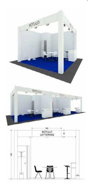
**GUIDING DRAWING:** It is not permitted to pierce or nail elements to the stand. It shall be adapted to the dimensions of the space allocated.
