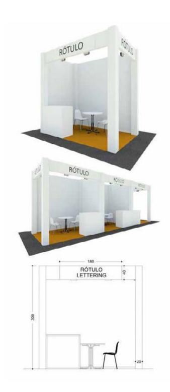
**GUIDING DRAWING:** It is not permitted to pierce or nail elements to the stand. It shall be adapted to the dimensions of the space allocated.
